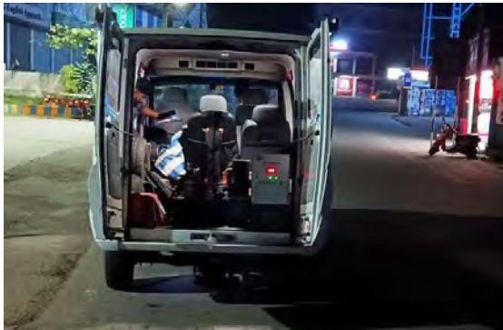
FWD Test at Peerumedu Devikulam Road
