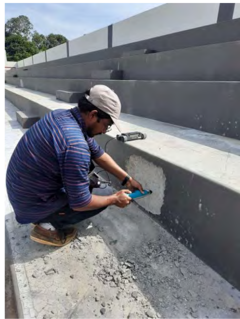
Rebar locator and Rebound Hammer Test at Thanur Stadium
